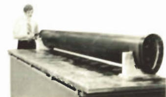
Submarine radome housing for sensitive radar equipment, receiving final inspection for service on a U.S. Navy vessel.
