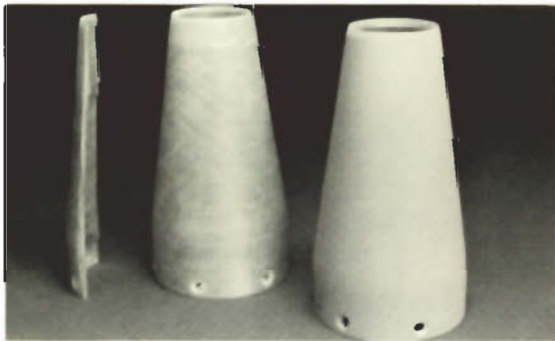
Lightweight filament wound nose cone for the AIM-9 Sidewinder missile.
